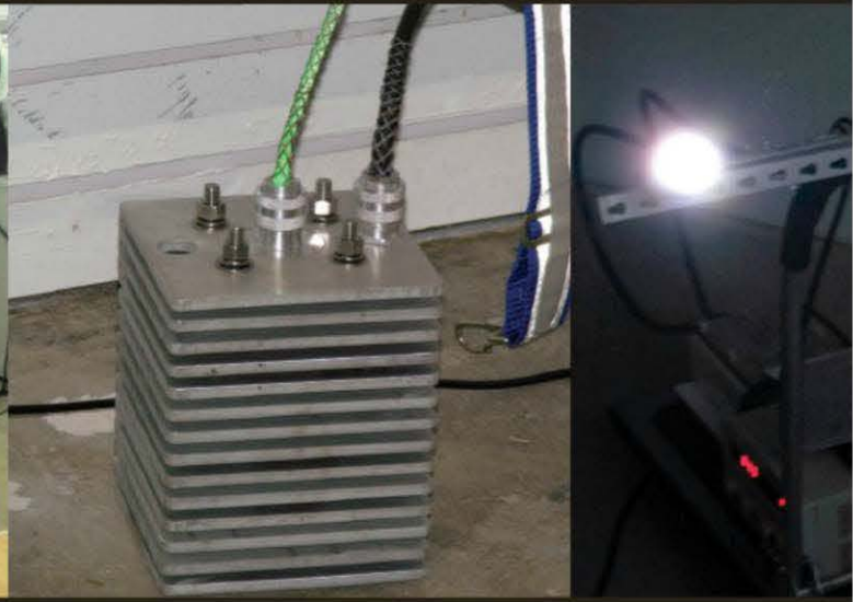
The illuminator in an MSHA approved blast proof box
